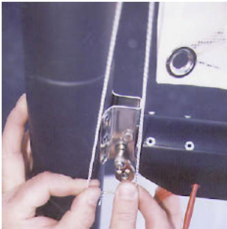
the head of the bolt and the cheek block on the starboard side of the gooseneck. This will keep the halyard from swinging loose. Bunch up the halyard (if you don't coil it, the rope
