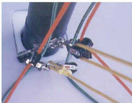
mounted on the deck behind the mast, tying it off between the cunningham blocks as above. The third part of the vang is the deck control line. It starts in the middle side deck clam cleat, goes forward to the remaining free block UNDER the outhaul line then up to the block on part two (the free block in the top picture), then back down repeating the pattern to the opposite side deck. The drawing shows the vang system without any other lines.
