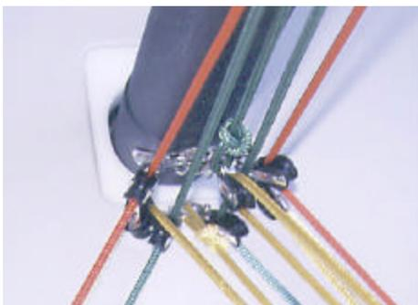
Slip the bungee loop up against the vang key to stop it falling out when close hauled.
