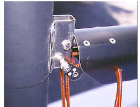
ends of the outhaul rope through the small blocks on the gooseneck and down to the TOP mini blocks which are attached on each side of the spar at the lower fitting. See below. From there, take them back to the TOP clamcleat on the deck and reattach the balls. Undo the temporary knot at the end of the boom and this completes the outhaul.
