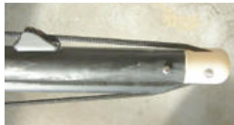
rope for securing it later. Make sure the bungee is in FRONT of the sheave before you tie on the sail so that you do not have to pull the bungee through the sheave. Properly rigged, it looks like the photo above. Tip: Do not pull up and jam the sail at the top. You need a little slack to be able to release from the clamcleat.
