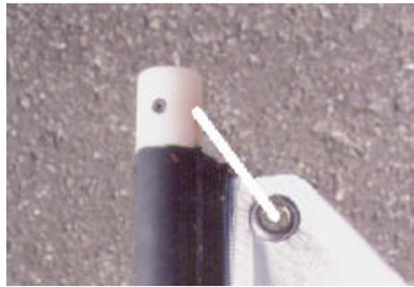
top, the angle at which the halyard pulls gets close to 45° which makes the last few inches of hoisting quite hard. There is a small piece of bungee passed through the halyard
