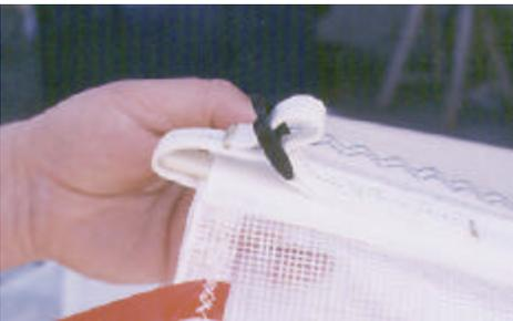
At the back end of the batten, pass the webbing over the batten and through the buckle as shown and tighten until snug. Do not overtighten or you will induce too much bend in the batten and the sail will be too full in light air.
