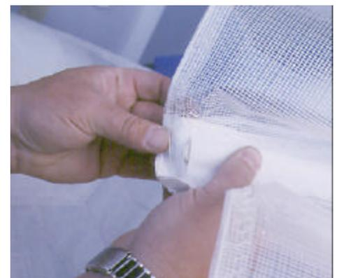
The top batten is a "full length" batten and does not have any elastic at the front end. Instead there is a batten
