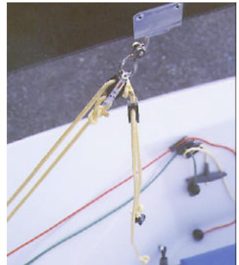
Attach the single block with becket, twist shackle and vang key into the slot of the boom key plate. That finishes the first part - the second part is shown hanging above. One
